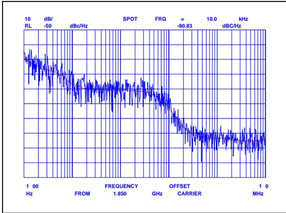
Figure 1. SKY72300 Main Synthesizer Phase Noise at 1850 MHz
