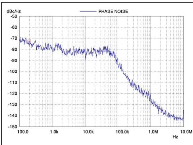
Figure 3. SKY74038 RF Synthesizer Phase Noise at 2380 MHz
