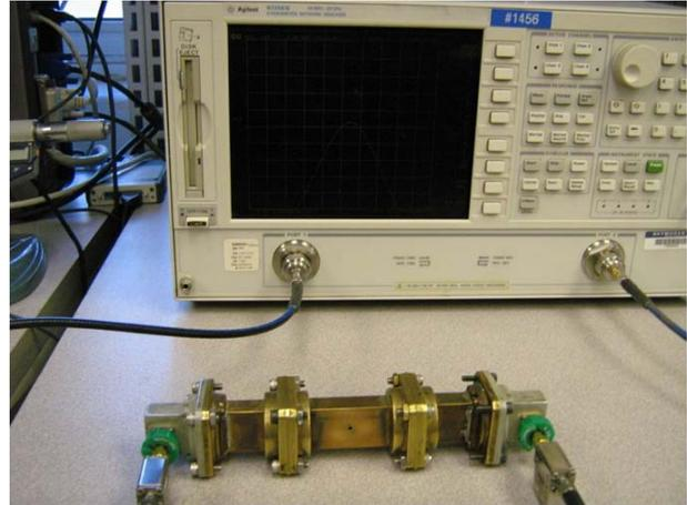
**Figure 1. Typical TE<sub>103</sub> Cavity Resonant at 9300 MHz**
